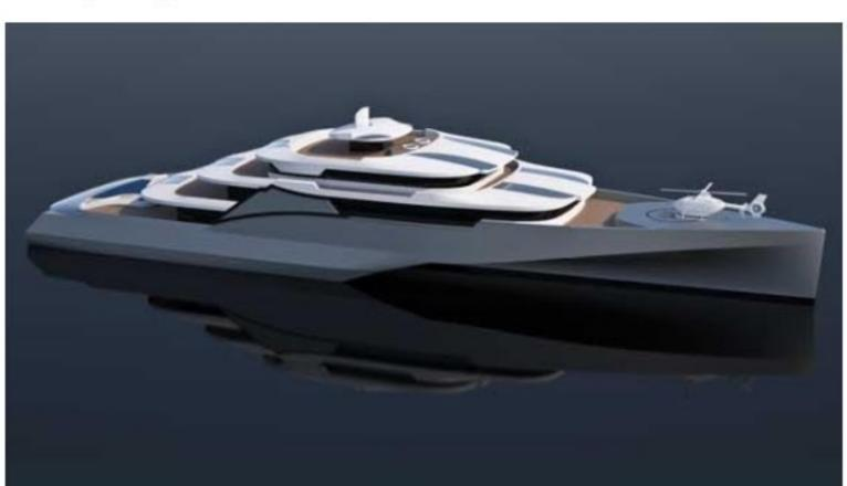
Australian designer Misha Merzliakov has penned a 102m trimaran based on a fast, efficient, seasickness-banishing hullform by the shipbuilder Austal.
