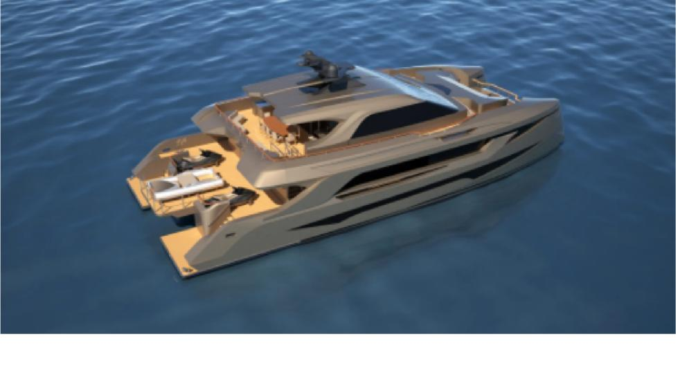
Also aft, a hydraulically lowering swim platform can be used to launch and retrieve the tender as well as delivering guests safely into the water for swimming, diving and other water sports.
